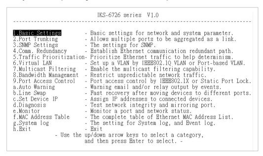
7. Use the following keys on your keyboard to navigate the Moxa switch's serial console:
