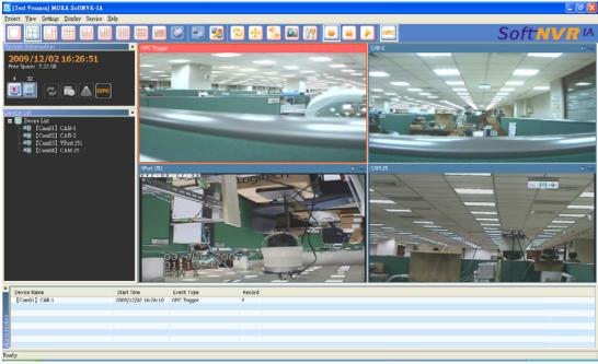
Step 5: To disable this OPC Trigger, click on the mouse's right button on the video image and select the "Alarm Confirmed" in the this menu.
