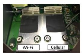
2. Insert the wireless module in the designated socket and tighten the two screws on the module.
