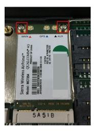
3. Attach the flat end of the antenna cable to the connector marked MAIN on the module. Follow the procedure described above to attach the AUX antenna cable.
