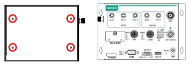
Fasten the screws to the back panel of the UC-8540
