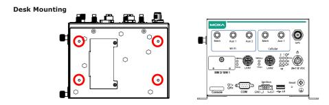
Fasten the screws to the bottom panel of the UC-8540
