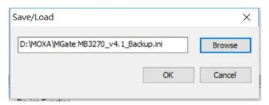
Wait for the MGate Manager to finish configuring the target device. If you import the configuration file successfully, a confirmation message will pop up. After closing the message dialog, the MGate Manager will automatically execute a Broadcast Search for all MGate units on the LAN. Your MGate should reappear in the list of units.
