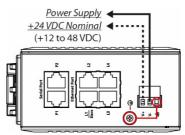
**NOTE** You should install the wiring for the power input terminal block using 20-12 AWG (0.5-3.31 mm2), applying a torque value of 7 lb-in and stripping the wire length to 4-5 mm.
