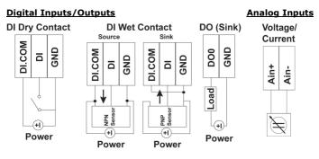
NOTE Install the wiring for IO terminal blocks using 22-16 AWG (0.32-1.31 mm2), a torque value of 3 lb-in, and a wire strip length of 5.5-6.5 mm.
