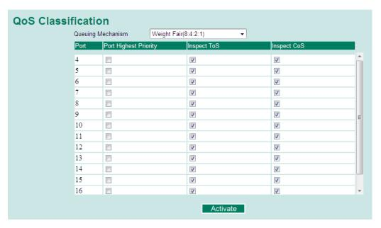
The TN-5500 supports inspection of layer 3 TOS and/or layer 2 CoS tag information to determine how to classify traffic packets.
