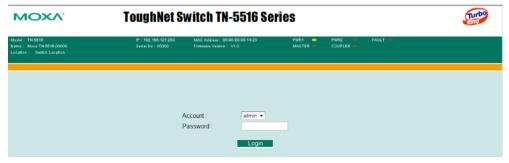
**NOTE** By default, no password is assigned to the TN-5500's web, serial, and Telnet consoles.
