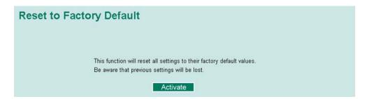
This function provides users with a quick way of restoring the TN-5500's configuration to factory defaults. This function is available in the serial, Telnet, and web consoles.
