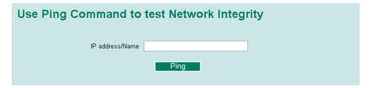
The **Ping** function uses the *ping* command to give users a simple but powerful tool for troubleshooting network problems. The function's most unique feature is that even though the ping command is entered from the user's PC keyboard, the actual ping command originates from TN-5500 itself. In this way, the user can essentially sit on top of TN-5500 and send ping commands out through its ports.
