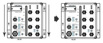
**NOTE** To provide greater protection from vibrations and shocks, use screws with shaft diameter between 6.0 mm and 7.0 mm, and fix the ToughNet switch onto the wall directly through the large opening of the keyhole-shaped apertures.
