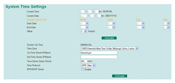
The Moxa switch has a time calibration function based on information from an NTP server or user specified time and date. Functions such as automatic warning emails can therefore include time and date stamp.
