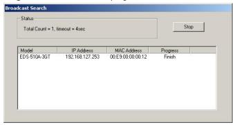
2. Once the search is complete, the Configurator window will display a list of all switches that were located.
