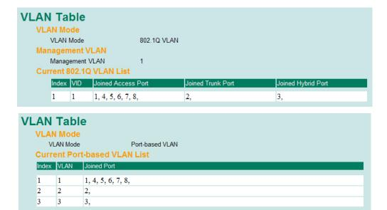
Use the **802.1Q VLAN table** to review the VLAN groups that were created, **Joined Access Ports**, **Trunk Ports**, and **Hybrid Ports**, and use the **Port-based VLAN table** to review the VLAN group and **Joined Ports**.
