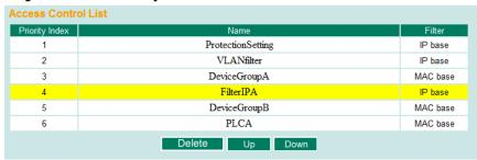
Changing an established access control list's priority is easy. Moxa provides a simple interface to let you easily adjust priority. Follow the three steps below to adjust the priority:
