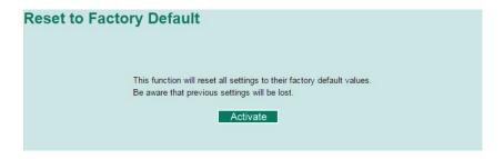
This function provides users with a quick way of restoring the Moxa switch's configuration to factory defaults. The function is available in the serial, Telnet, and web consoles.
