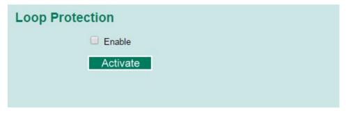
Check the Enable box and click Activate to enable the Loop protection.
