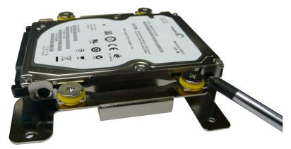
4. When finished, place the bracket on the computer, and use four screws to fasten the bracket. Next, find the location of the power connect and the SATA connectors. There is one power connector which can be used by two SATA hard disks, and there are two SATA connectors for connecting two SATA disks.
