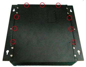
4. Then remove seven screws on the rear cover.
