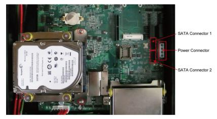
5. Connect the power cable to the power connector and the SATA cable to the SATA connector.
