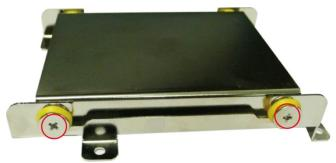
3. Place the hard disk on the bracket. Use the four screws to fasten the hard disk at both sides of the bracket.
