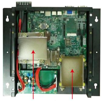
First HDD Bracket Second HDD Bracket
