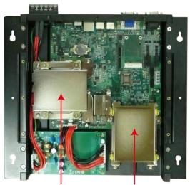
First HDD Bracket Second HDD Bracket
