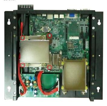
7. After the first HDD bracket has been removed, you can find two memory modules. Carefully remove the module by clicking the clutches at both sides of the module, and then replace the new module. Be sure to orient the module correctly.
