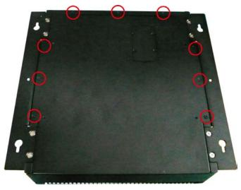
3. Then remove seven screws on the rear cover.
