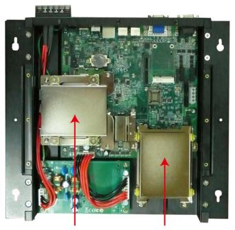
First HDD Bracket Second HDD Bracket
