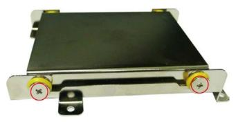
3. Place the hard disk on the bracket. Use the four screws to fasten the hard disk at both sides of the bracket.
