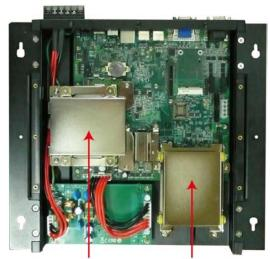
First HDD Bracket Second HDD Bracket
