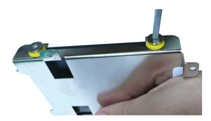
4. When finished, place the bracket on the computer, and use four screws to fasten the bracket. Next, connect the SATA cable to the SATA connector, and the power cable to the power connector.
