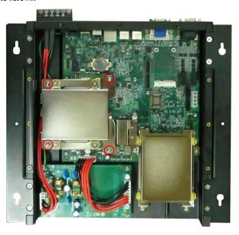
6. After the first HDD bracket has been removed, you can find two memory modules. Carefully remove the module by clicking the clutches at both sides of the module, and then replace the new module. Be sure to orient the module correctly.
