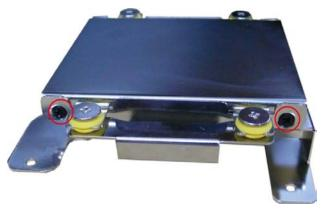
3. Place the hard disk on the bracket. Use the four screws to fasten the hard disk at both sides of the bracket.
