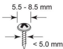
Do not drive the screws in all the way into the wall—leave a space of about 2 mm to allow room to slide the wall-mounting kit between the wall and the screws.
