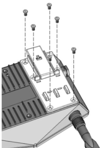
The **DK-DC50131** die-cast metal kit can be bought separately, and enable easy and robust installation for the AWK-6222. A pair of DK-DC50131s is needed for DIN-rail mounting. To install the DIN-rail mounting kits, tightly attach the two DIN-rail mounting kits on the rear panel of AWK-6222 with 12 screws (6 screws for each kit).
