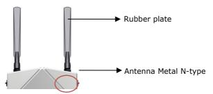
Step 1: Use your fingers and hold the antenna metal N-type connector.
