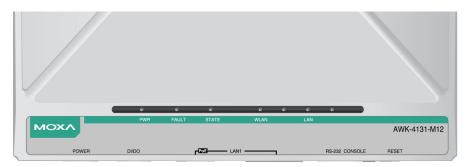
The following table is a summary for the wireless settings and LED displays. You can check the status of the AWK-4131 by reading these LEDs. More information about "Basic Wireless Settings" is presented in Chapter 3.
