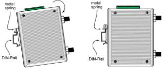
To remove the AWK-3121-M12 from the DIN-Rail, simply reverse Steps 1 and 2.
