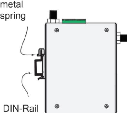
To remove the AWK-1121 from the DIN rail, simply reverse Steps 1 and 2.
