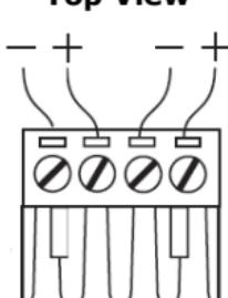
**STEP 2:** To keep the DC wires from pulling loose, use a small flat-blade screwdriver to tighten the wire-clamp screws on the front of the terminal block connector.
