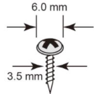
Do not drive the screws in all the way into the wall—leave a space of about 2 mm to allow room for sliding the wall mount panel between the wall and the screws.
