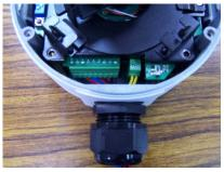
**NOTE** Be sure to arrange the cables carefully to make sure that all cables are connected properly. We recommend connecting the Ethernet cable first, and then the 9-pin terminal block. Connect the 2-pin terminal block last.
