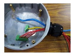
**NOTE** When installing the cable gland, make sure the 2 rubber rings are assembled properly for IP66 protection. If necessary, use silicon sealant.
