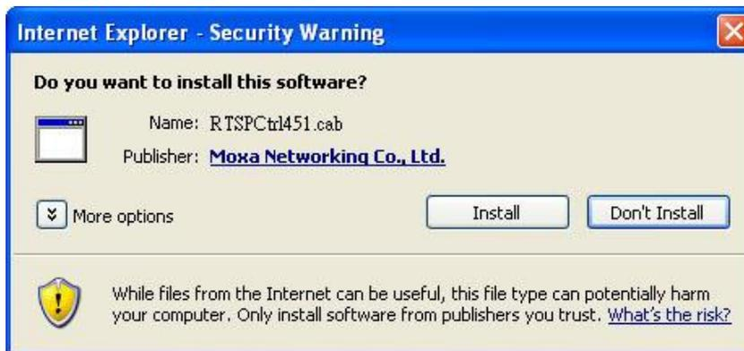
**NOTE** For Windows XP SP2 or above operating systems, the ActiveX Control component will be blocked for system security reasons. In this case, the VPort's security warning message window may not appear. Users should unblock the ActiveX control function or disable the security configuration to enable the installation of VPort's ActiveX Control component.
