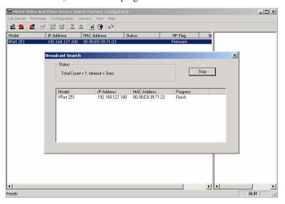
3. When the search has concluded, the Model Name, MAC address, IP address of the EDS Switch and VPort will be listed in the Utility window.
