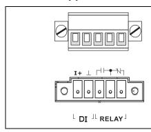
**STEP 1:** Insert the negative (ground)/positive DI wires into the  $\frac{\perp}{11}$  terminals.
