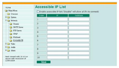
Accessible IP Settings allow you to add or remove "Legal" remote host IP addresses to prevent unauthorized access. Access to the VPort is controlled by IP address. That is, if a host's IP address is in the accessible IP table, then the host will be allowed access to the VPort. Administrators can allow one of the following cases by setting this parameter:
