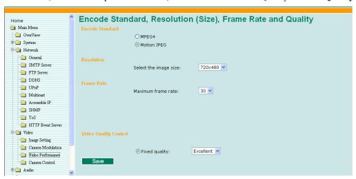
For MPEG4, users can setup **Resolution, Frame Rate** and Video Quality in **Fixed Bit Rate** or **Fixed Quality**.
