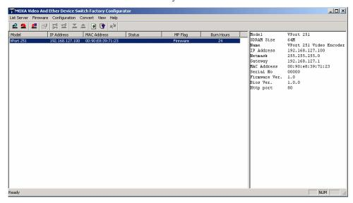
The **Broadcast Search** only can search the devices on the same domain LAN. If your devices are located on different domain LAN, you can use the **Specify IP Address** to search the device by key in the IP address.
