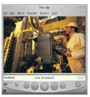
The video performance of the VPort 251 in other media players may not always be the same. For example, you will notice a greater delay when viewing the VPort 251's video from QuickTime player compared to viewing it directly from the VPort 251's built-in web server. In addition, viewing the VPort 251's video from Quicktime player through a router or Internet gateway could result in a broken connection.
