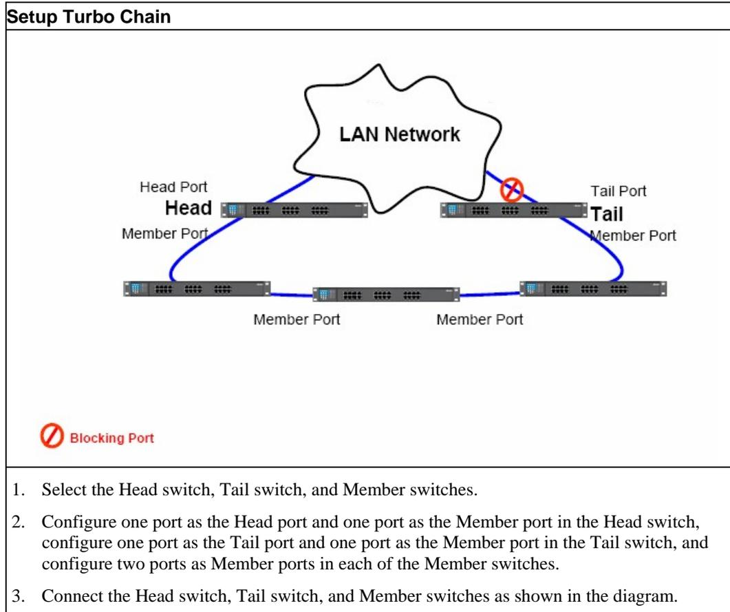
The path connecting to the Head port is the main path, and the path connecting to the Tail port is the back up path of the Turbo Chain. Under normal conditions, packets are transmitted through the Head Port to the LAN Network. If any Turbo Chain path is disconnected, the Tail Port will be activated to continue packet transmission.
