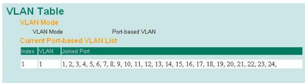
In 802.1Q VLAN table, you can review the VLAN groups that were created, Joined Access Ports, and Trunk Ports, and in Port-based VLAN table, you can review the VLAN group and Joined port.
