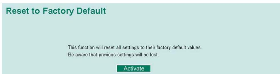
This function provides users with a quick way of restoring the IKS-6500's configuration to factory defaults. This function is available in the serial, Telnet, and web consoles.
