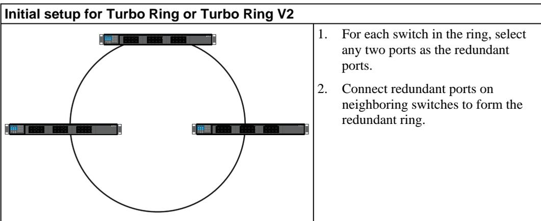
The user does not need to manually assign the master with Turbo Ring or Turbo Ring V2. If no switch is assigned as the master, the protocol automatically selects one of the switches to be the master. The master is only used to identify which segment in the redundant ring acts as the backup path. In the following subsections, we explain how the redundant path is selected for rings configured for Turbo Ring and Turbo Ring V2.
