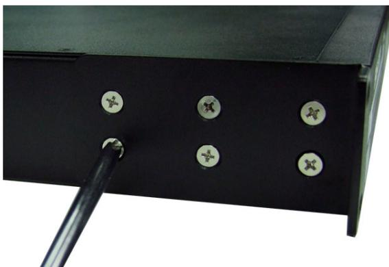
**Step 3: Installing the SMG-6100 to a rack.**
