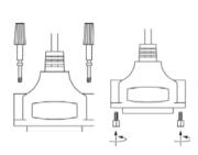
\* Connect to Female \* Connect to Male Connector Connector
