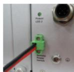
**Step 4:** Connect the earth/ground cable to the Phillips-head ground connector on the lower right corner of the front panel.
