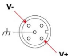
**Step 5:** Connect the power cable (CBL-Power Jack to M12) to the M12 (A-coded, 5-pin, male) connector as shown at right. Then connect the power connector to power input 1 on the front panel.
