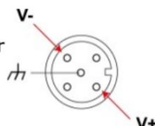
**Step 5:** Connect the M12 connector to the power source using the pin assignment at right.
