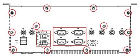
3. Remove the cover of the rear panel, and disconnect the internal power connector.
