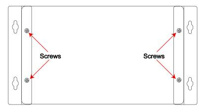
Step 2: Use two screws per side to attach the V2406-24I to a wall or cabinet.
