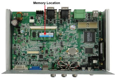
5. Carefully remove the module by pushing the latches on both sides of the module, and then replace the new module. Be sure to orient the module correctly.
