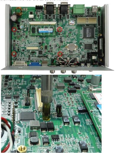
8. Place the HDD bracket onto the mainboard of the computer, and then fasten the bracket with the screws.
