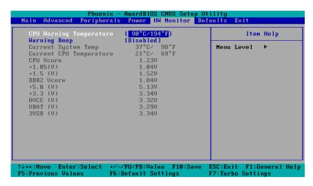
This item helps monitor the status of the system, including CPU temperature and the voltage of the CPU, SDRAM and battery.
