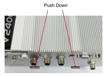
To re-install the computer on the DIN-rail, use a screwdriver to press the buckle so that it can be released. Now, it can be re-installed on the DIN-rail.
