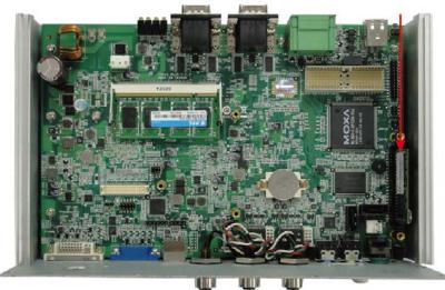
2. Pull up and take off the DOM module, and then place the new DOM module into the slot.
