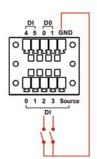
**DI Wet Contact Wiring**
