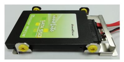
6. Place the hard drive disk on the bracket, and then use the screws to fasten.
