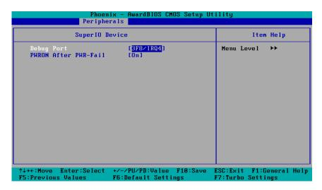
This function allows you to enable/disable the debug port communication. The V2406-24I computer will automatically distribute the IRQ value for the debug port as the default value. If you wish to disable, select **Disabled**. This port is only for engineers who are debugging programs.
