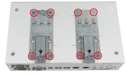
When the brackets are firmly attached with the screws, it can be installed on a DIN-rail
