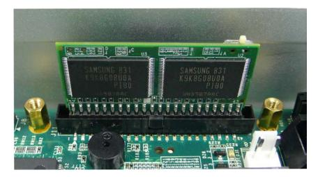
Insert the new DOM module; make sure it is firmly inserted.
