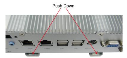
To re-install the computer on the DIN-rail, use a screwdriver to press the buckle so that it can be released. Now, it can be re-installed on the DIN-rail.
