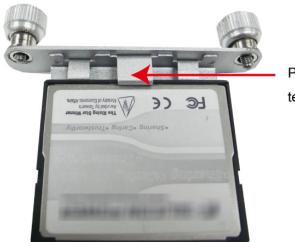
Put CF Card into tenon/hook of CF socket
