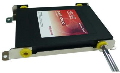
4. When finished, place the bracket on the main board and find the location for attachment.
