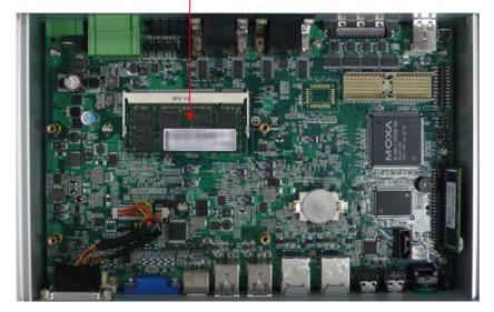
Carefully remove the module by clicking the clutches at both sides of the module, and then replace the new module. Be sure to orient the module correctly.
