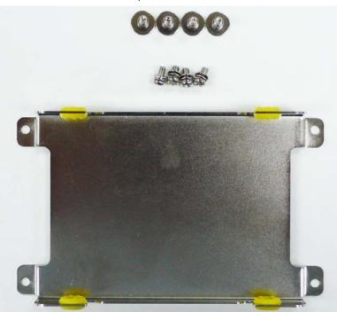
3. Place the hard drive disk on the bracket and use four screw to attach it.
