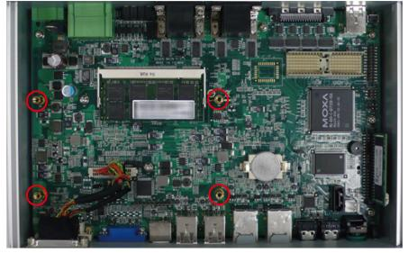
5. Make sure that four screws have been securely attached on the main board. Then use the SATA cable to connect the hard drive disk to the SATA connector, and use the power cable to connect to the power connector.
