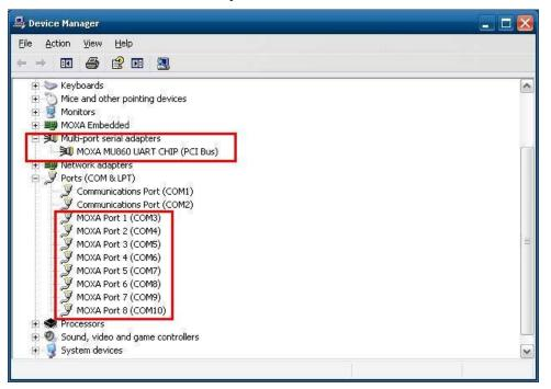
Right-click the **MOXA MU860 UART CHIP (PCI Bus)** and select **Properties** to re-assign the port number for each COM port.
