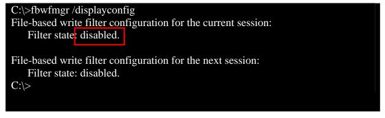
2. Type **fbwfmgr** /enable to enable FBWF. Reboot the system for the changes to come into effect.
