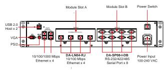
**NOTE**: Expansion modules can be installed in either Slot A or Slot B. For example, in the above figure the LAN port module DA-LN04-RJ is installed in Slot A and the serial port module DA-SP08-I-DB is installed in Slot B.
