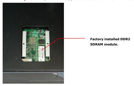
4. Carefully remove and replace the memory module. Be sure to orient the module correctly.
