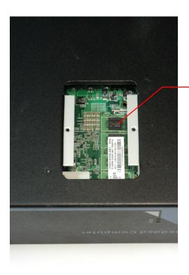
Orient the memory module correctly
