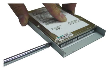
5. Next, install the SATA hard disk and hard disk bracket back into the DA-682.
