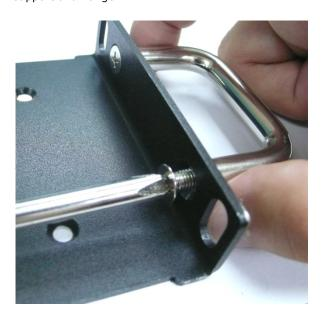
Step 3: Installing the rackmount ears to the DA-682.
