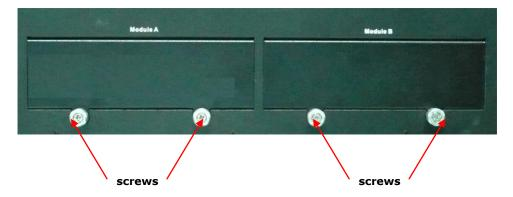
3. Carefully insert or remove the expansion module by pushing or pulling on the two screws at the same time. By pushing or pulling on the two screws evenly, you can ensure that the board is inserted or removed without being damaged.
