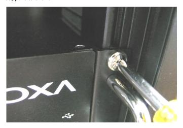
Note that four screws are required to attach the DA-682 to the rack. Use two screws on the left side and two screws on the right side.
