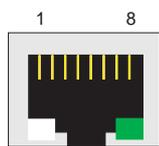
The bottom right corner LED indicator maintains a solid green color when the cable is properly connected to a 100 Mbps Ethernet network. The LED will flash on and off when Ethernet packets are being transmitted or received.
