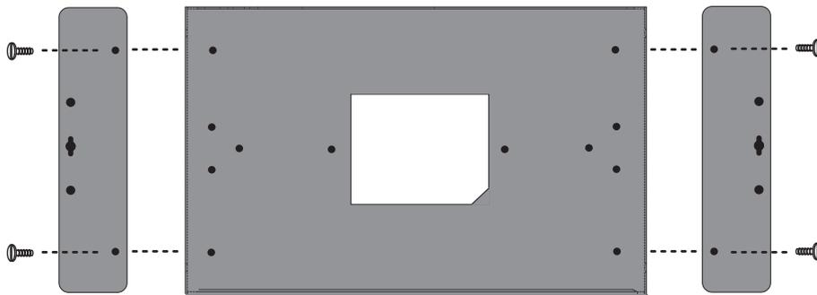
Figure A: UC-7408 Universal Communicator—Wall Mounting Brackets (bottom view)
