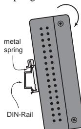
**STEP 2:** The DIN-Rail attachment unit will snap into place as shown below.
