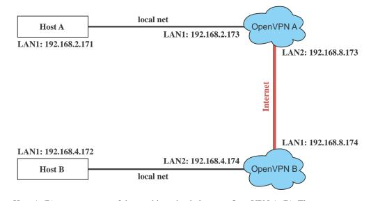
1. Set up four machines, as shown in the following diagram.
