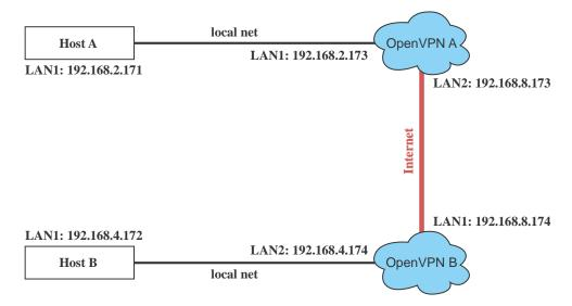
2. The configuration procedure is almost the same as for the previous example. The only difference is that you will need to comment out the parameter "up" in "/etc/openvpn/tap0-br.conf" and "/etc/openvpn/tap0-br.conf".
