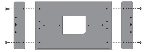
Figure A: UC-7402 Universal Communicator—Wall Mounting Brackets (bottom view)
