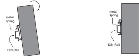
To remove the UC-8410/8416/8418/8430 from the DIN-Rail, reverse Steps 1 and 2 above.
