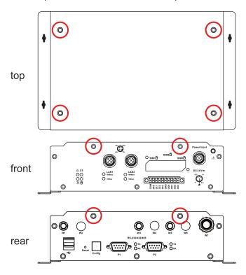
Only after removing all eight screws can you remove the top cover. One Wi-Fi module and one cellular module are pre-installed on the UC-8481's mini PCIe sockets. There are two more slots available for additional modules. Please note that Cellular Socket 2 can only accommodate a Cinterion PH8 cellular module, while either only a Wi-Fi or only a cellular module may occupy the remaining slot ("Socket 2").
