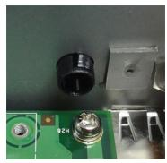
6. Remove the nut and locking washer from the threaded antenna connector.
