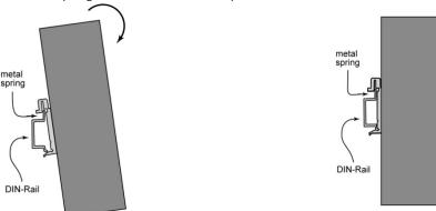
To remove the UC-8481 from the DIN rail, simply reverse Steps 1 and 2.
