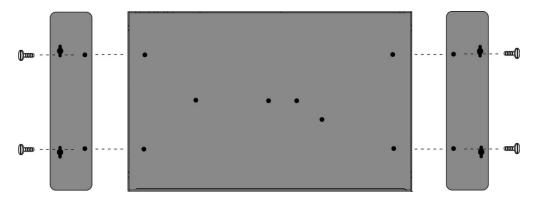
Figure A: UC-8481 Embedded Computer—Wall Mounting Assembly (bottom view)
