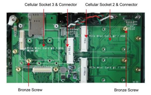
3. Install the cellular module into the socket by fastening the black screw into the standoff, at the end of the module.
