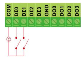
Note: If are using wet contacts, you must connect "COM" to power.
