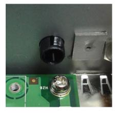
5. Remove the nut and locking washer from the threaded antenna connector.
