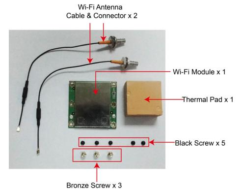
1. To install the module, first find the locations of the antenna connectors and connect the antenna cables to the module. Please note that there are two antenna cables on each side of the module.
