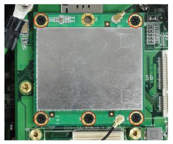
5. Connect the Wi-Fi module antenna connectors by using the W2 and W4 holes on the rear panel of the computer. Remove the antenna hole protection cover first.
