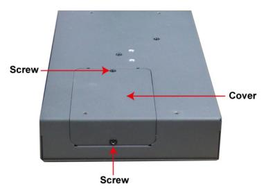
The CF is located on the motherboard beneath the cover at the back of the UC-8481. Use a screwdriver to remove the cover and access the slot. See the following figure for the locations of the CF socket.
