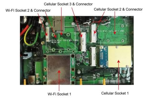
Please note that the cellular sockets are USB interfaces across Mini PCIe connectors; it is also possible to purchase Wi-Fi modules that use the same interface (mini PCIe with USB interface) for installation on the cellular sockets.
