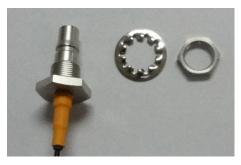
6. Pass the antenna mount's threaded connection ring through the mounting hole; keeping the locking washer against the rear panel face, secure the antenna connector by by tightening the provided nut onto the threaded protection ring.
