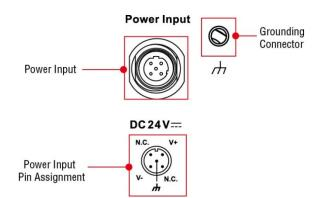
**SG:** The *Shielded Ground* (sometimes called *Protected Ground*) contact is the middle contact of the 5-pin power connector when viewed from the angle shown here. Or you may use the independent grounding connector beside the power input. Connect the SG wire to an appropriate grounded metal surface.
