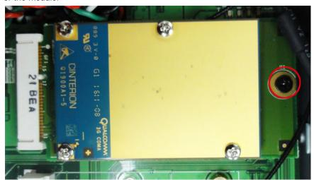
4. Connect the cellular module antenna connectors to either the W2 or W4 hole on the rear panel of the computer. First, remove the antenna hole protection cover.
