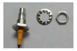
7. Pass the antenna mount's threaded connection ring through the mounting hole; keeping the locking washer against the rear panel face, secure the antenna connector by by tightening the provided nut onto the threaded protection ring.
