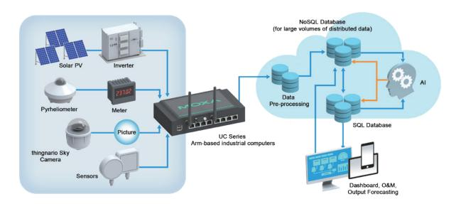
The technology produced by thingnario was designed to capture all of the data from the inverter as well as weather data from their self-developed Sky Camera, which provides information about cloud coverage and how the solar panels will be affected.
