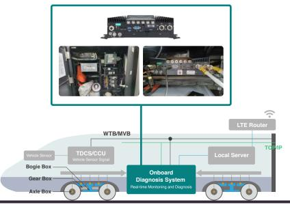
The onboard diagnostic system powered by Globiz's CBM utilizes Moxa's computer to enable edge computing.
